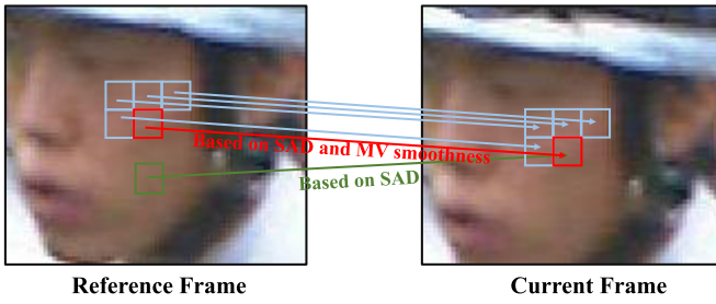
Fig. 4. This figure illustrates the MV generated based only on SAD constraint, and the MV generated based on the integration of SAD and MV smoothness constraints. Sole reliance on SAD may result in inaccurate results. However, by imposing constraints on the smoothness of the MV, the correct MV can be determined.
