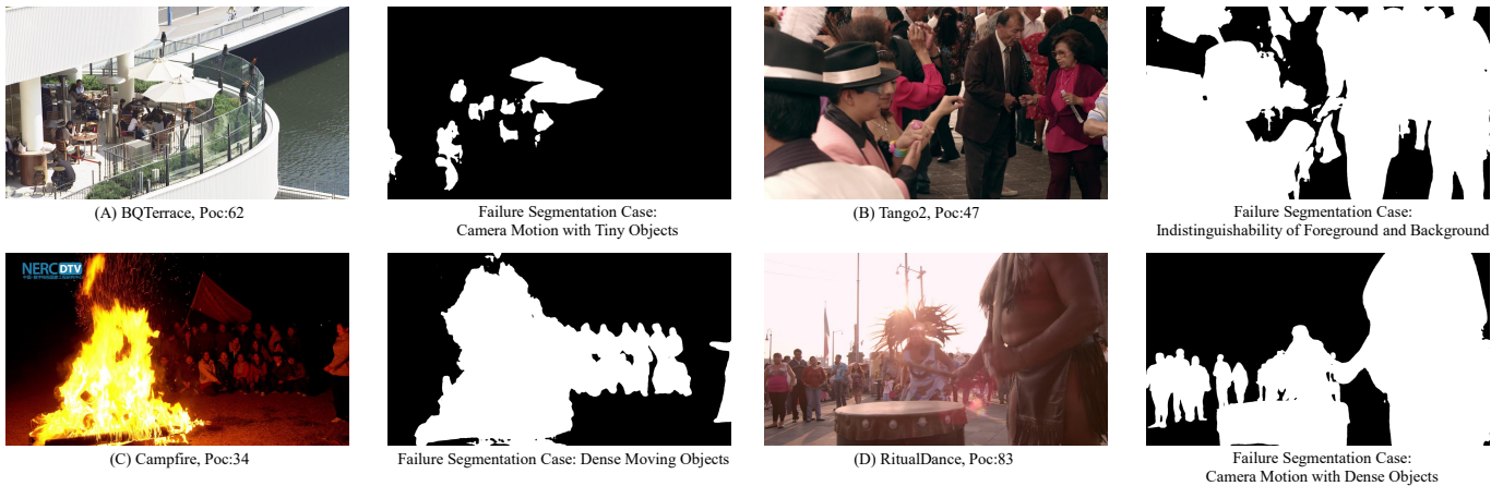
Fig. 2. Failure segmentation cases on some sequences with special cases (extreme motion, serious occlusion, large resolution).
