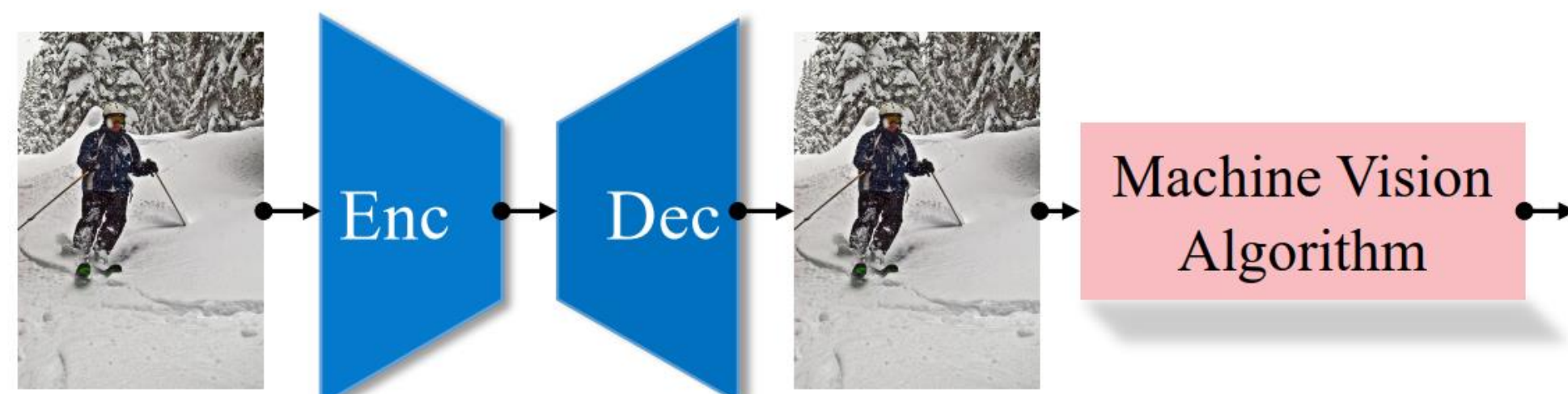
(a) First type of joint optimization: Machine vision algorithm is applied on the reconstructed image.
