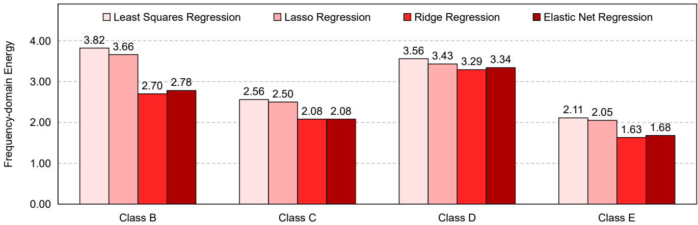
Fig. 5. The average frequency-domain energy of residuals obtained with different solvers. Candidate model solutions include least squares regression, lasso regression, ridge regression, and elastic net regression.
