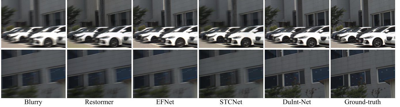
Fig. 9. Visual comparison on the REVD dataset. Compared to advanced motion deblurring methods, DuInt-Net restores fine textures more accurately, preserving details such as vehicle edges and window frames. Please zoom in for better visualization.
